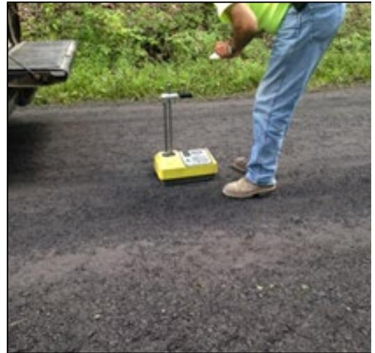
**Figure 17.** Compaction Testing with Nuclear Density Gauge
