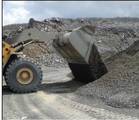
**Figure 2.** Laying out the sampling pile
