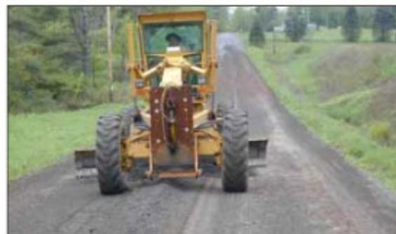
**Figure 29.** Material is knocked down
