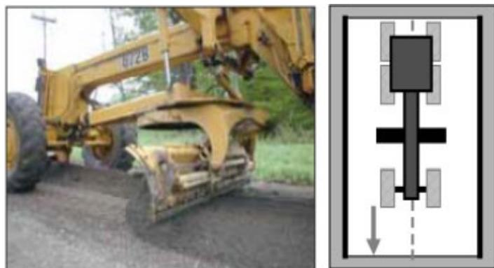
**Figure 30.** Grader leaving the road with a high flat center.
