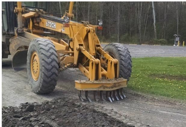
**Figure 26.** Grader equipped with scarifier teeth.
