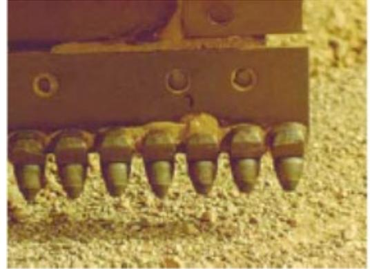
**Figure 21.** Individual carbide steel cutting bits
